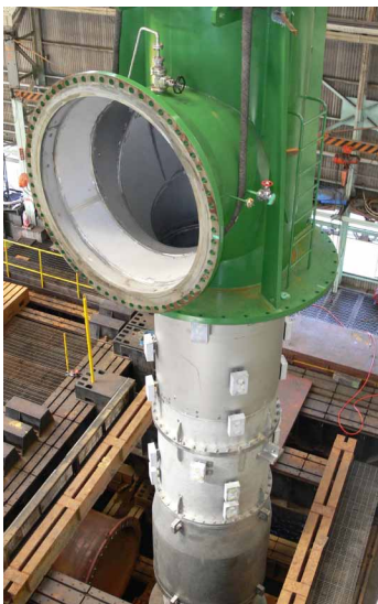
Main Cooling Water Pumps 29,500m 3 /h - 20m - 2,400kW - 2units
