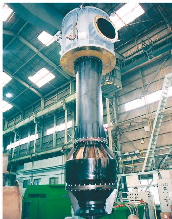
Brine recirculation pump for Sabia MSF desalination plant, Kuwait (Size:1000mm, Driver:3550kW)
