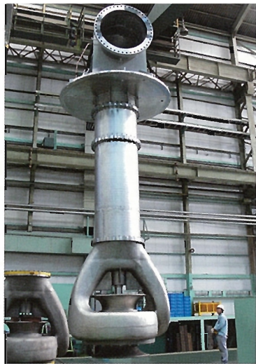
Brine recirculation pump for Jebel Ali M (MSF) desalination plant, U.A.E. (Size : 1,200mm, Driver : 4,900kW)
