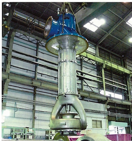
Brine recirculation pump for Shuweiht S2 IWPP (MSF) desalination plant, U.A.E. (Size : 1,200mm, Driver : 4,100kW)
