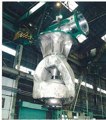
Hot well pump for Darajat III Geothermal power station, Indonesia (Size : 1,200mm, Driver : 1,050kW)
