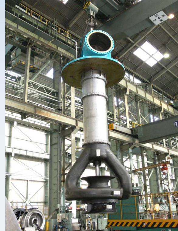
The same type as being installed as a main pump in Dubai
